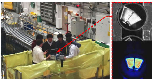
▲ Cherenkov light measurement (ATR) to check nuclear materials from spent fuel
